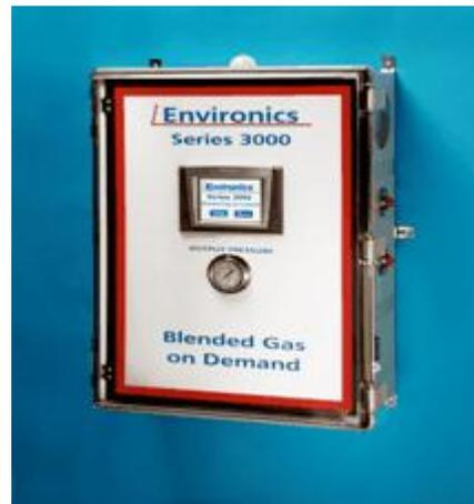
The system is manufactured in a NEMA 4 wall mount enclosure, with internal electrically grounded aluminum panels for support and a clear polycarbonate door to protect the controls. Optional enclosures are available. Fitting connections and tubing are 316 stainless steel.
